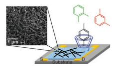
Nanotube detects isomers: A chemiresistive material based on carbon nanotubes wrapped with a calixarene-substituted polythiophene displays a selective and sensitive response to xylene isomers (see picture), as demonstrated by conductance changes, quartz crystal microbalance, and fluorescence studies. This demonstrates the promise of low-cost, real-time sensors utilizing host-guest chemistry.
